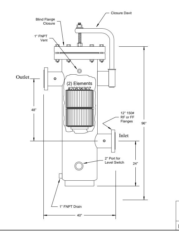
**FilterFab** MANUFACTURING CORPORATION MODEL C12-285F COALESCING FILTER
